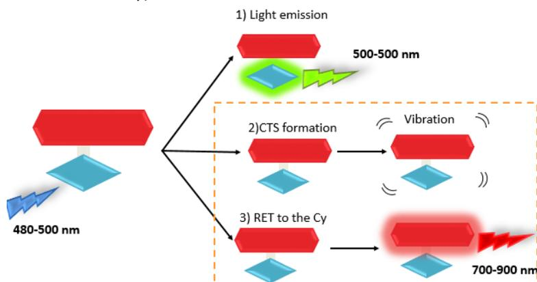
After making the measurements, it is possible to make a proportion between the BODIPY fluorescence (used as reference, due to its viscosity independence) and the Cyanine fluorescence (conditioned to the viscosity).
